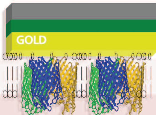
Diagram demonstrating the structural features of the device with the OmpF and lipids adsorbed to the gold electrode surface. The neutron beam passes through the magnetic reference layer (green) prior to and after reflecting from the device interface.
