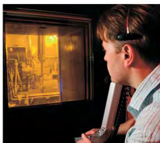
◀ Final preparations being made on the new tungsten neutron target and reflector assembly prior to its first operational run in May. This work was undertaken within the remote handling cell via two pairs of master/slave manipulator arms positioned either side of the target and moderator assembly. 09EC2037
