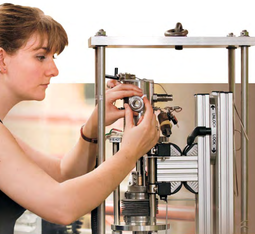
◀ Sarah Rogers (ISIS) preparing the new Loq pressure cell. 08EC2300 The graph shows small angle scattering profiles of dry (blue circles) and hydrated micelles (yellow circles) stabilised in sc -CO 2 by the surfactant TC14. The scattering obtained (triangles) when using the surfactant AOT 4 is also shown for comparison. The inset shows a schematic representation of a hydrated reverse micelle in sc -CO 2 .
