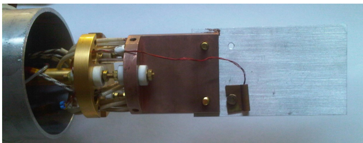
CCR cold head showing the “floating” Cernox thermometer attached to a sample plate (back view)
