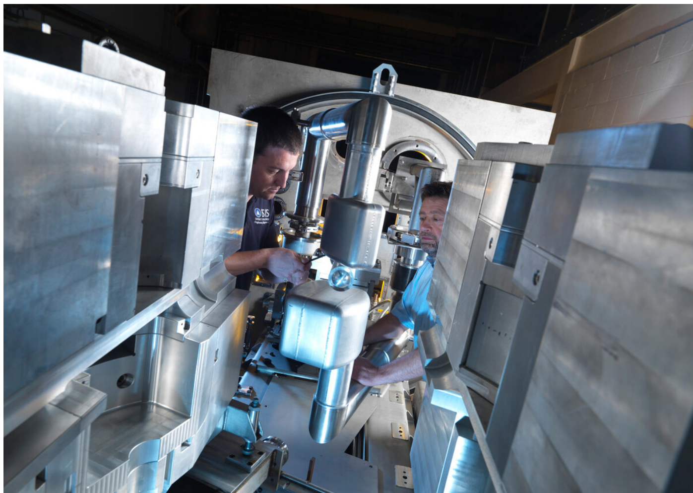
Andy Robinson and Chris Russell check dimensions on Target Station 2's mock up target, reflector and moderator system. The reflector is open to reveal the target in the centre and the moderators above and below.
