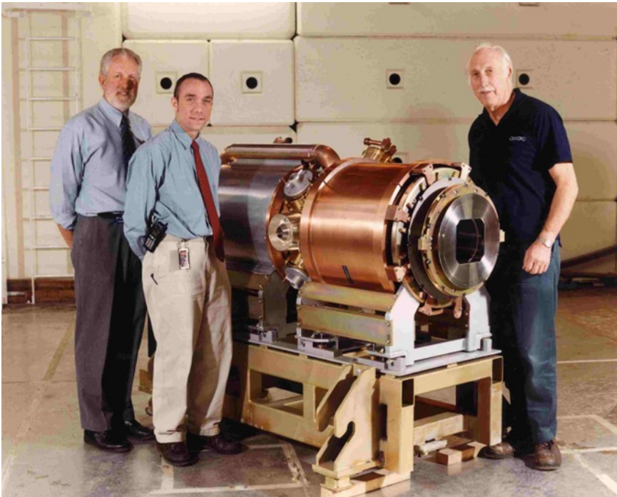
In 2004, ISIS began to install a 'second harmonic' system to increase the amount of beam to accelerate. Here, design engineers John Hirst, David Jenkins and technician Terry Western inspect one of the four systems before installation.
