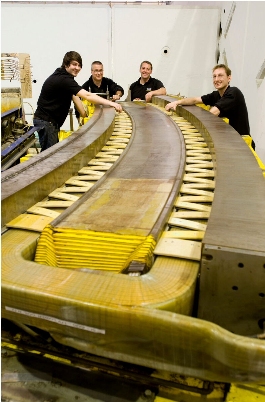
Left to right: Jamie Searis, Steve Cook, Adrian Hooper and Oliver Newell, of the Accelerator Engineering Group, at work on the lower half of one of ISIS's dipole magnets as it is refurbished in July 2011.
