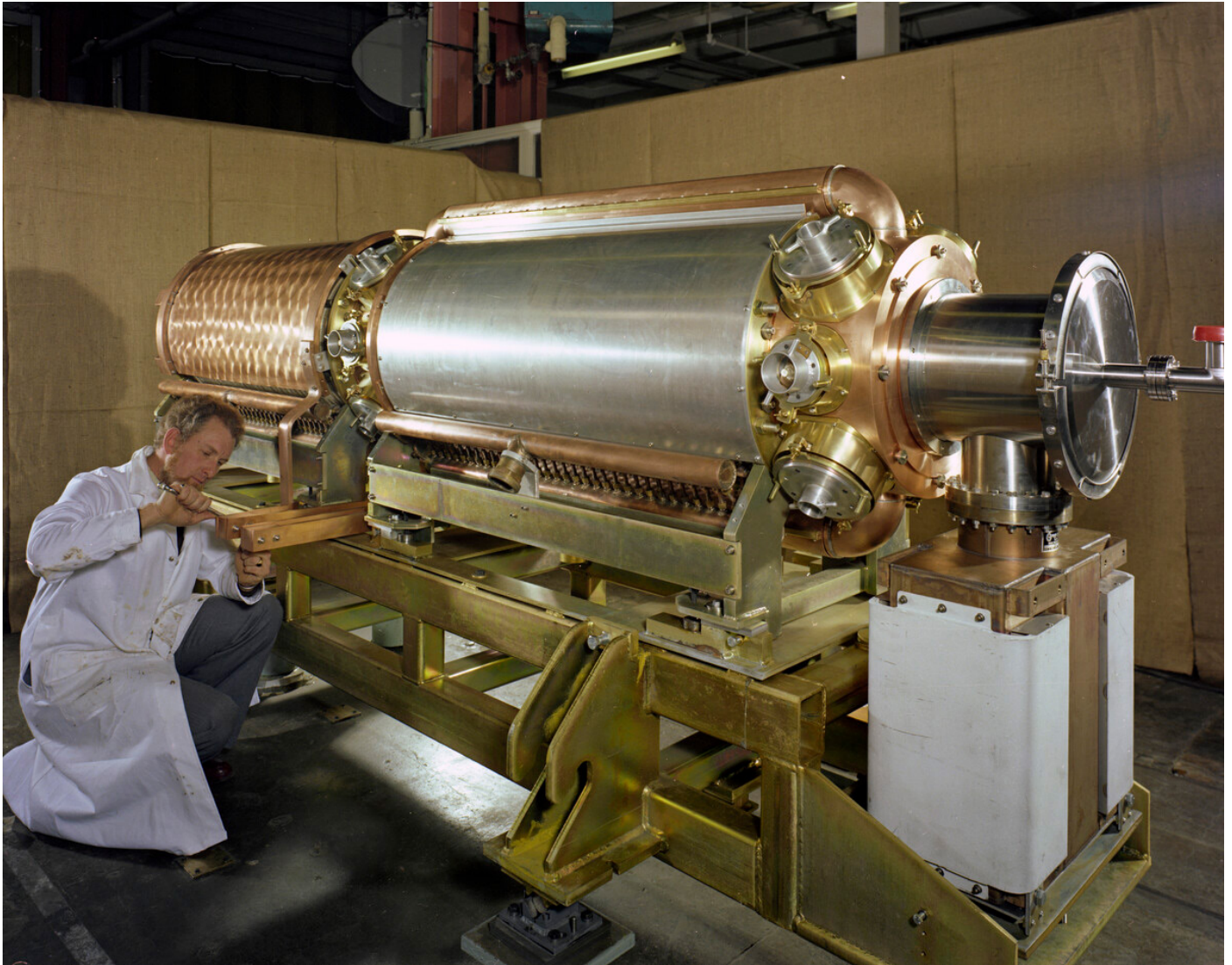
Design engineer John Hirst preparing one of the first ISIS radio-frequency cavities in March 1982. These are the systems that accelerate the protons in the synchrotron.
