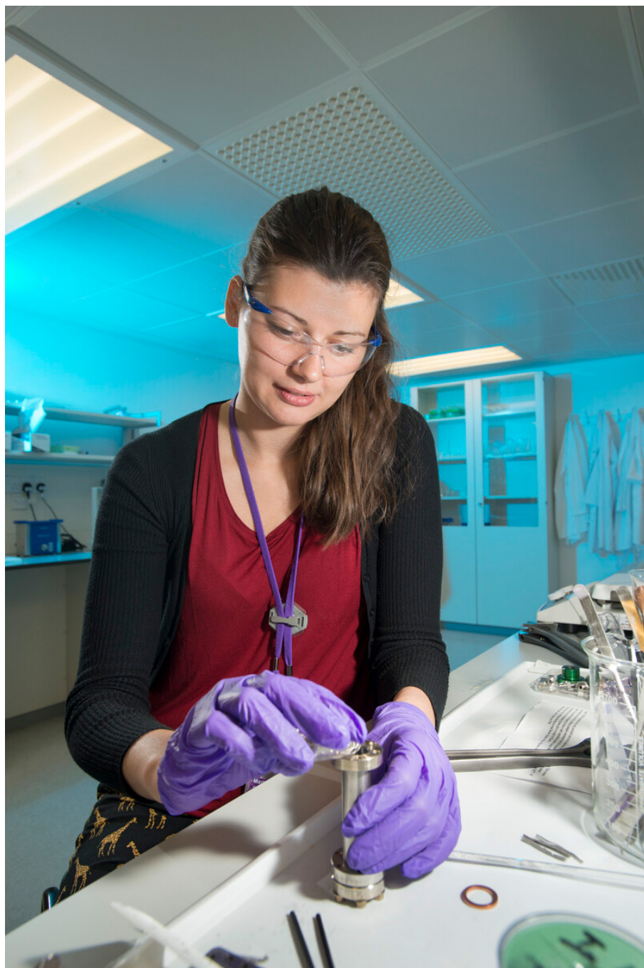
Marta Falkowska, University of Manchester, prepares samples for studies of catalytic arene hydrogenation on Nimrod in 2014. Catalytic hydrogenation is an important reaction for the synthesis of many compounds used in the chemical, pharmaceutical and food industries.
