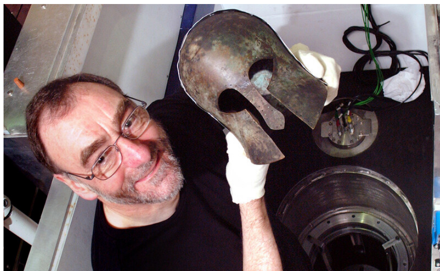
A 2500-year-old Corinthian-type bronze helmet being put into position on ROTAX by Roy Garner, The Manchester Museum, in 2003. Measurements revealed a different bronze composition of the noseguard compared with the rest of the helmet, suggesting the noseguard was not part of the original structure.
